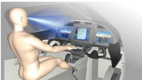
“At the same time, we were moving components around in CAD, using a digital human mannequin to learn what was possible, to establish a pilot’s eye point, hip point, reach zones, and sightlines.”
