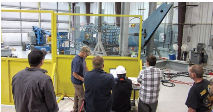
Pressure testing the fuselage at 18 psi - no problem!
