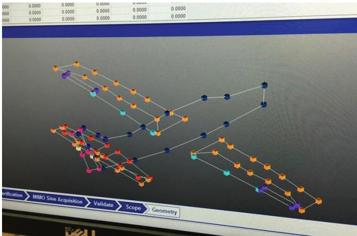
Attachment points for Ground Vibration Testing (GVT)
