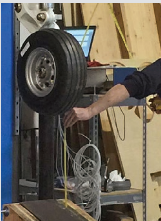
Main gear drop test
