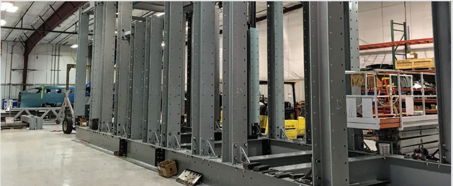
Structural test rig for fuselage and wing structural testing
