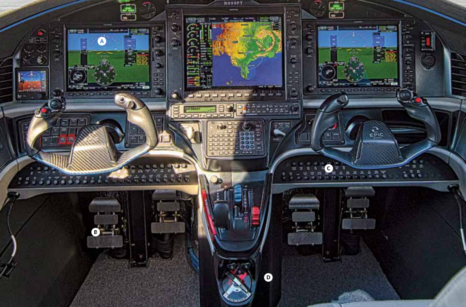
A The E1000 panel is dominated by Garmin's G1000 NXi, with two PFDS and a center-mounted MFD, providing the most-current avionics features available today.
