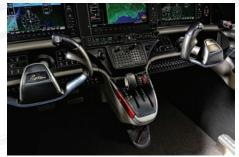
**CONSOLIDATED PILOT WORKFLOW** To enhance pilot work flow, the team focused on optimizing movement, reach and visibility. The E1000 flight deck is intuitive, effortless, with key flight management systems strategically positioned and sequenced logically to reduce arm movement, minimize fatigue, and avoid shadowing displays.
