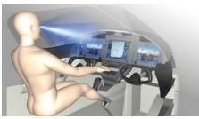
"At the same time, we were moving components around in CAD, using a digital human mannequin to learn what was possible, to establish a pilot's eye point, hip point, reach zones, and sightlines."
