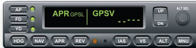
Figure 3: Track VDI within 5% of GP or 10 seconds elapses (GPSV)
